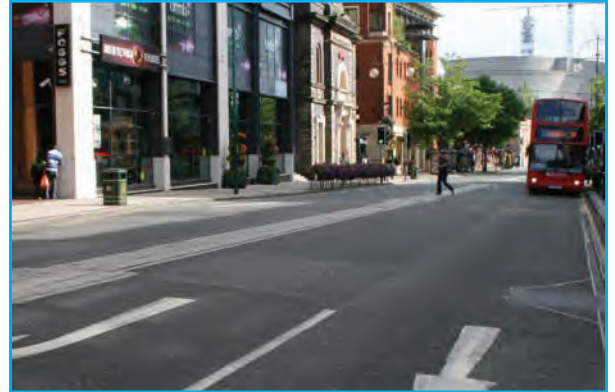
This informal median on Broad Street, Birmingham has operated successfully for many years
