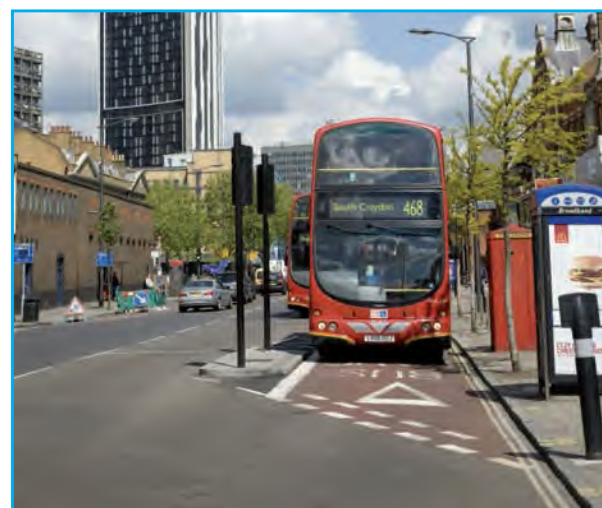
Bus Advance Area, Walworth Road MPR scheme
